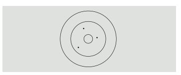
The second target has three shots that are scattered around the center. These are not precise. If you average all of the shots, the accuracy would be right on the bull's eye. But if you are only going to make one measurement, you want that one measurement to be accurate. Without good precision you will not always have accurate results.
