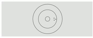
Using a target as an example, accuracy is how close your shot is to the center of the bull's eye. The three shots on the target are close to the center but a little biased to the right. "Bias" is a word used to describe or indicate how far you are from the "true" value or the bull's eye. For comparison purposes, the "true" value may be a well standardized reference method or the result you get from the method you currently use.
